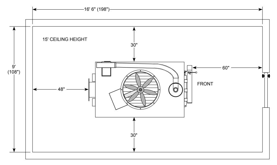
ROOM SHOULD BE INSULATED AND HAVE RETURN AIR FROM THE AREA TO BE HEATED. WHEN USED TO PROVIDE AIR MAKE UP FOR THE PLANT, ROOM MUST HAVE AN OUTSIDE AIR SOURCE.
