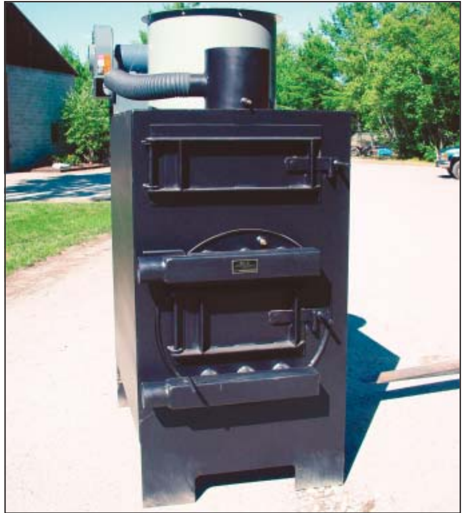
Peter C. Herman Inc. has four wood furnaces (similar to one above) from Biomass Combustion Systems; company burns its waste wood material for fuel.
